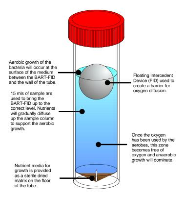
Sergei Winogradsky originally reported this type of phenomenon forming in waters kept in tall glass cylinders at the end of the nineteenth century. The beauty of this device is that different microbes prefer to function at different sites on the redox gradient and so can be seen being active and reacting within that zone. Very often, the first sign of this is the development of a cloud of growth that may be fuzzy and diffuse or a flat plate floating in the watery medium.
